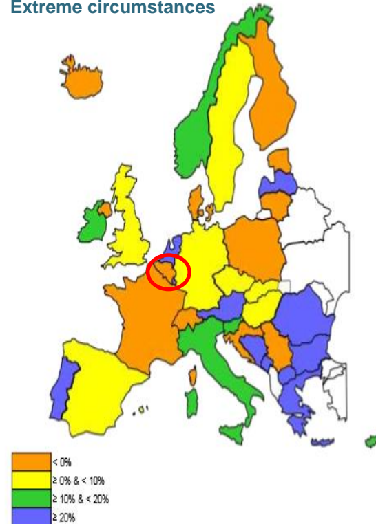
F 4.1.8 – Remaining Capacity minus Adequacy Reference Margin as a part of Reliably Available Capacity per country, Scenario B, January 2020, 7 p.m.
